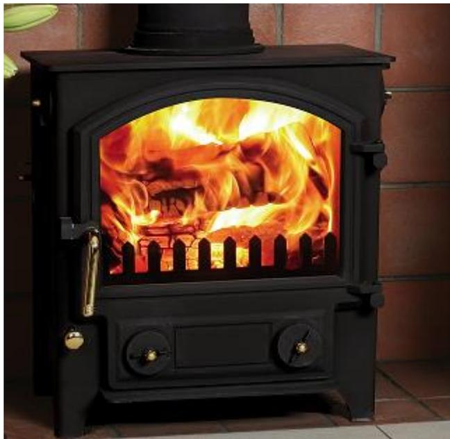
The Little Thurlow Smoke Control Eco stove has a nominal heat output of 5kW., and a weight of 61 kg. The flue gas mass flow is 4.3 g/s for wood logs, 3.7 g/s for solid fuel. The mean flue gas temperature directly downstream of the flue spigot at nominal heat output is 281 degrees C (wood) 276 degrees C (solid fuel). The stove is designed as a closed appliance and is capable of intermittent operation. Tested Net efficiency 79.0% (wood), 80.2% (solid fuel).
